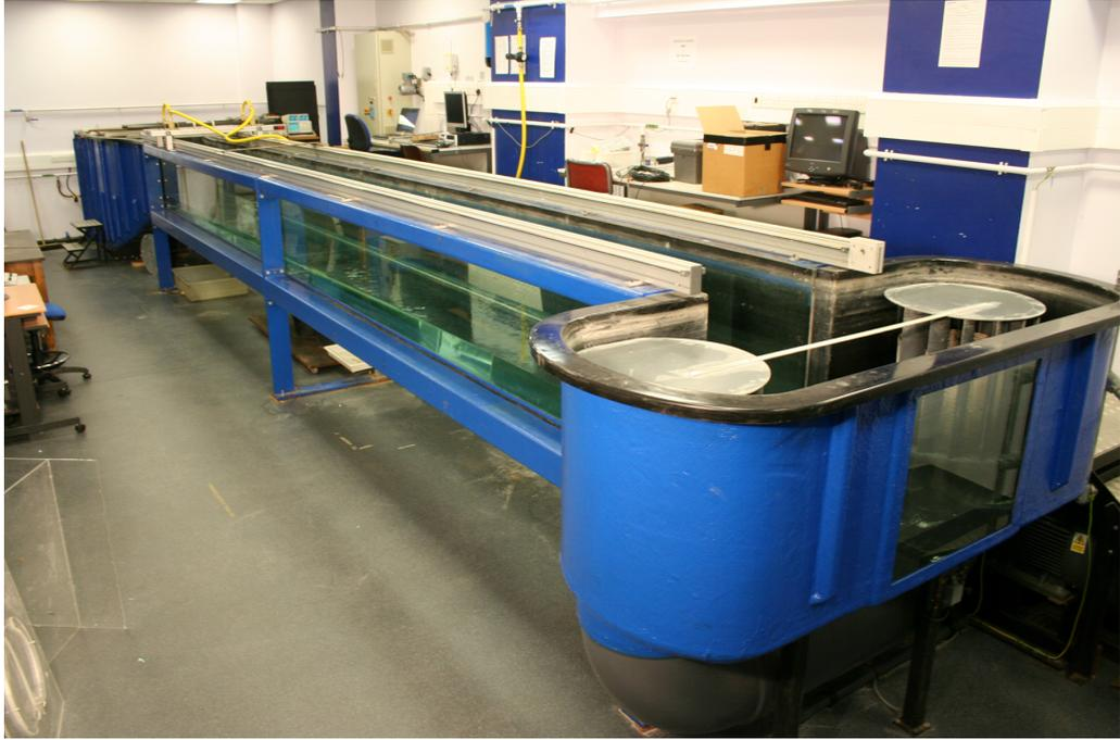
Fig. 4.1: Recirculating water channel at Imperial College London.
