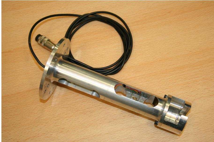
Fig. 4.7: Photograph of the load cell showing a pair of strain gauges installed on one of the webs.
